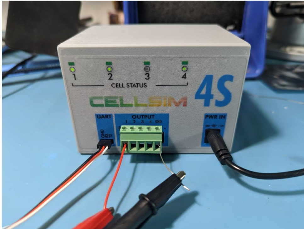
CELLSIM 4S connected to a load. Left: UART connection to master via USB-UART converter. Middle: OUTPUT connector with connections to DC load. Right: Power input barrel jack connector.
