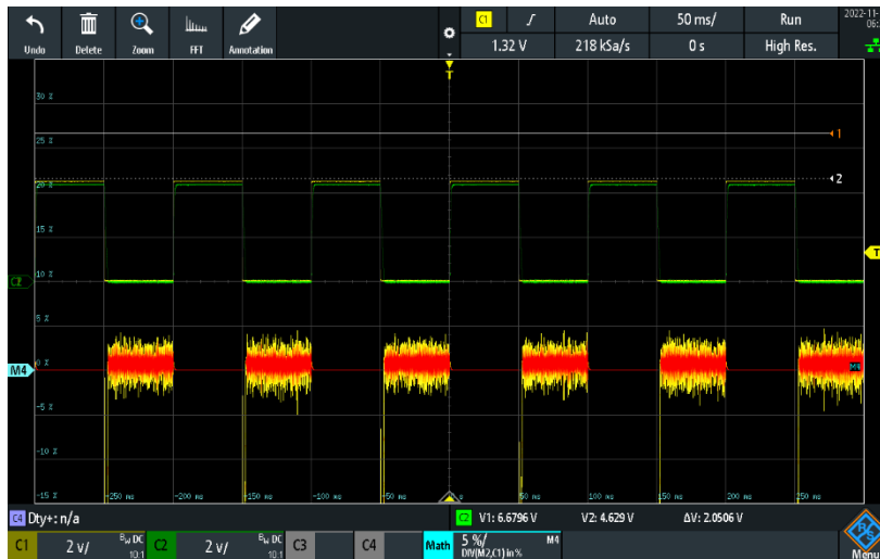
Output voltage percent error while tracking a 10Hz 0-4.5V square wave with a load current of 200mA on a DC electronic load. Error waveform shown in orange and yellow (bottom). Yellow waveform (CH1) is commanded output voltage, green waveform (CH2) is actual output voltage.
